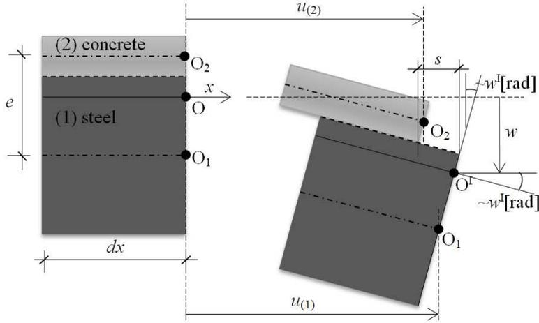
Fig.2: The slip in the contact of beam layers
