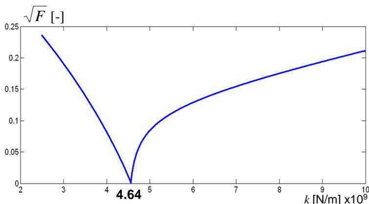
Fig.5: The diagram of square root of error function ( $\sqrt{F}$ ) in the dependence on shear stiffness  $k$  for the beam defined in the section 3
