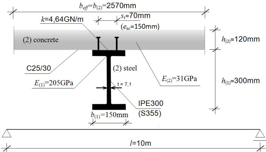
Fig.3: Cross-section and static scheme of the rib of analysed composite steel-ferroconcrete floor
