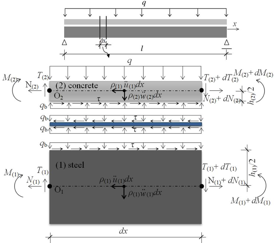
Fig.1: The static scheme of steel-ferroconcrete beam and its differential element with the forces acting over it
