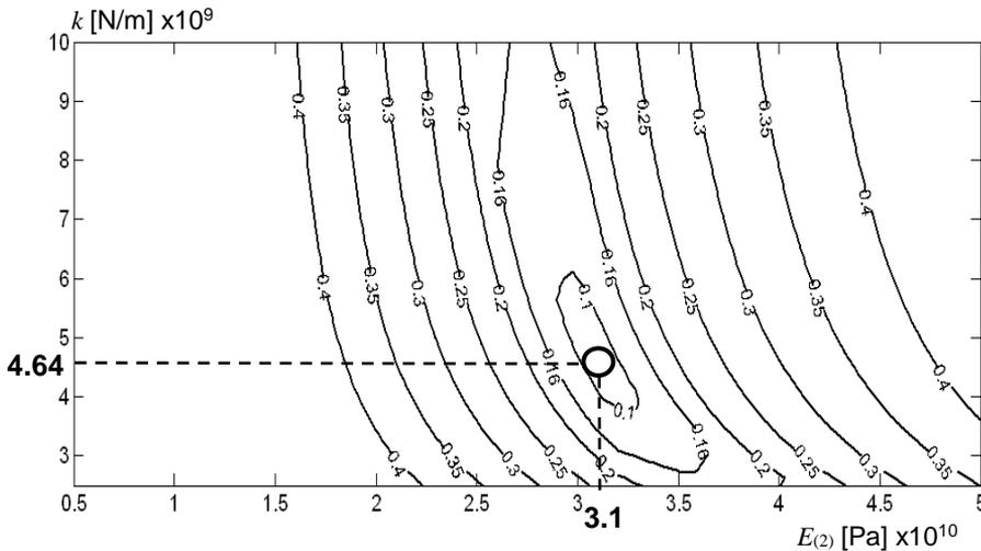
Fig.4: The contour line diagram of square root of error function (7<sub>1</sub>) in the dependence on shear stiffness  $k$  and Young' modulus of concrete plate  $E_{(2)}$  for the beam defined in the section 3
